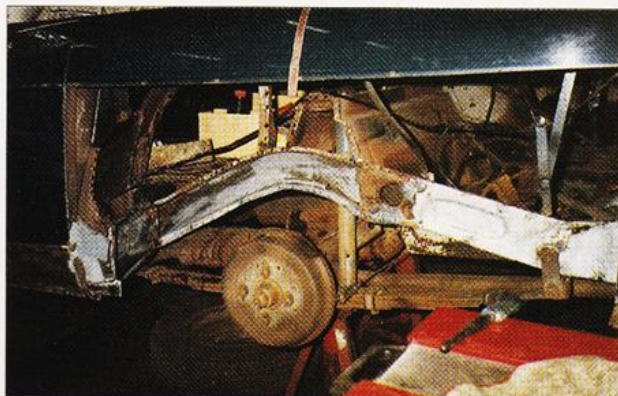
Lower rear wings were cut away. Both inner and outer rear wheelarches needed replacement
