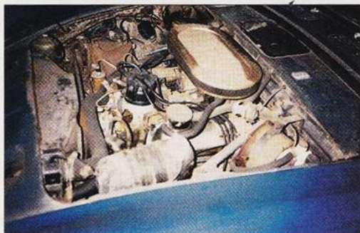
Left, the 4.2-litre small-block Ford V8 engine was seized solid after lying dormant for around 14 years
