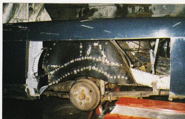
Lower rear wings were cut away. Both inner and outer rear wheelarches needed replacement
