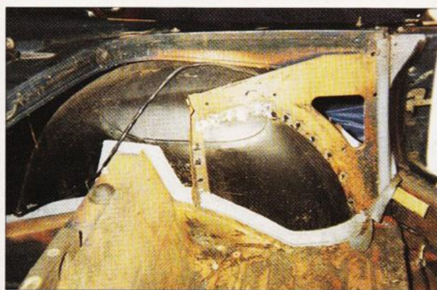
Below, the Tiger's rear wheelarches needed complete replacement
