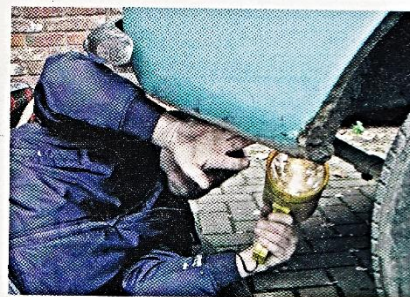
Base of each rear wing should have a drain hole – this one has been boded.
