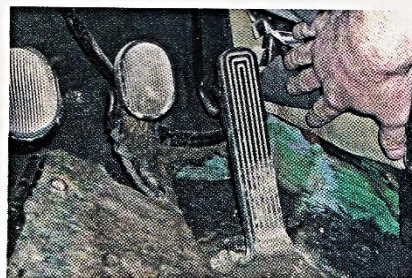
Footwells are rot-prone, especially the area around the accelerator pedal.
