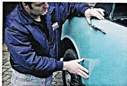
Check rigidity of structure by jacking up the car and looking at how the door shuts.
