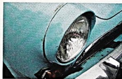
Area around headlamp is normally one of the first things to go – also check panel seams.
