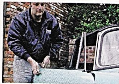
Door hinge pins are prone to wear as the doors are quite heavy, so check them.
