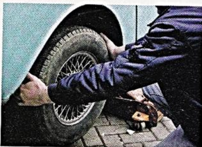
Check for worn splines and broken spokes if wire wheels are fitted on a well-used car.
