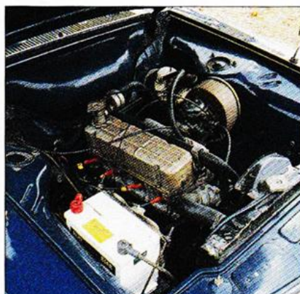
Only a single Stromberg carburettor for the Alpine, which loses out on performance.
