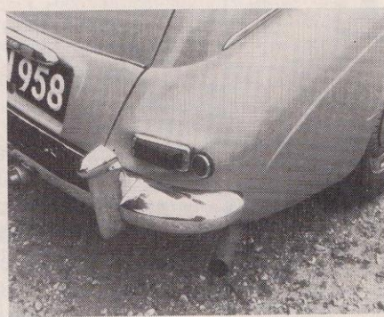
Below, areas to check for rusting; left, the forward edge of the rear wheel arch adjoining the door and right, where the rear bumper snuggles into the rear wing.
