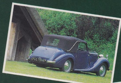
Above: Drophead always uses external pram-irons; bodies built by Abbot and (briefly) Carbodies. Right: Bakelite dash is same as introduced on Ten for '39 model
