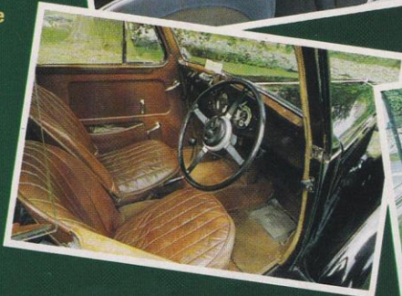
Right: Ten's gold-faced oval dial gave way in '38 to twin round dials; dash still timber
