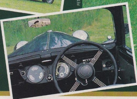
Above: Drophead always uses external pram-irons; bodies built by Abbot and (briefly) Carbodies. Right: Bakelite dash is same as introduced on Ten for '39 model
